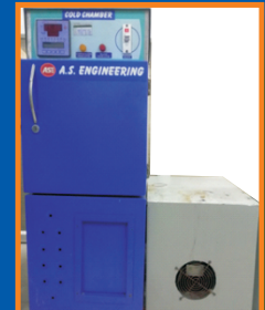
AGEING TEST IN CYCLE COLD/HOT CONDITION
