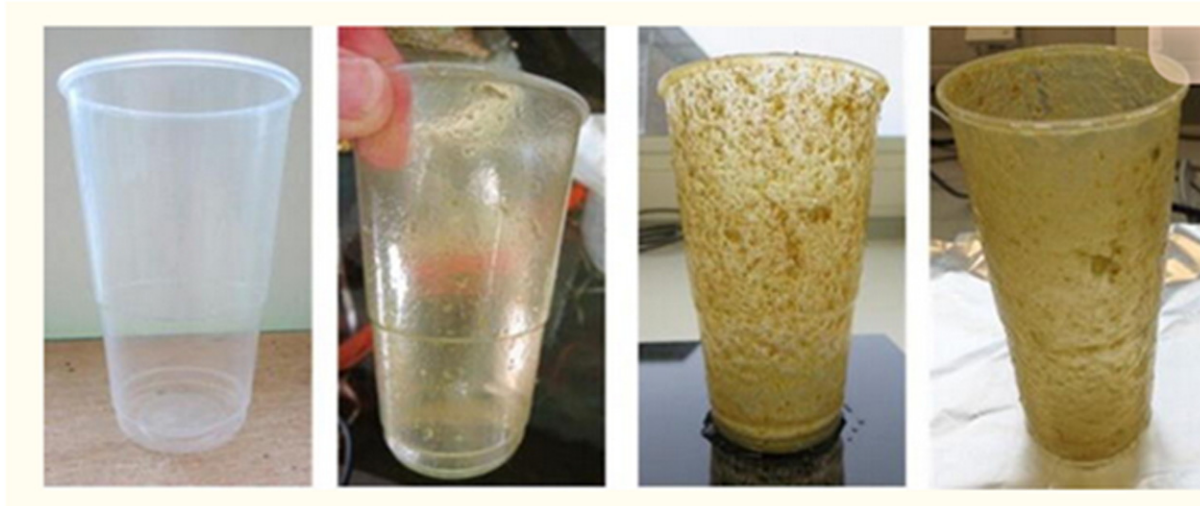
Fig. 4 Biofouling of polypropylene cup, after From left to right) 0, 57, 183 and 390 days in the microcosm, respectively. Reproduced from Gerritse, J., 2020. Fragmentation of plastic objects in a laboratory seawater microcosm. Sci. Rep. 10, 10945.
